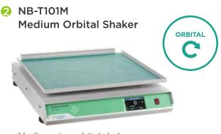
Medium size orbital shaker. Shaking up to  $5 \times 2L$  flasks or 20kg. Its low height & proper weight make shaking stable even with a heavy load.
