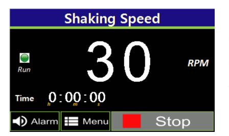
The 3.2 inch easy-to-read LCD touch screen displays shaking speed in RPM and timer to assure that the shaker is running according to the setting value and also it enables an user to adjust the values precisely even with gloved fingers.
