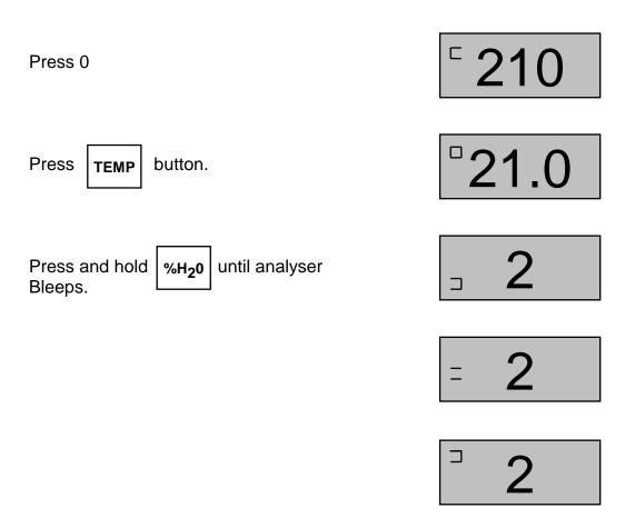
This completes the hardware resetting. Now check the temperature and capacitance readings.
