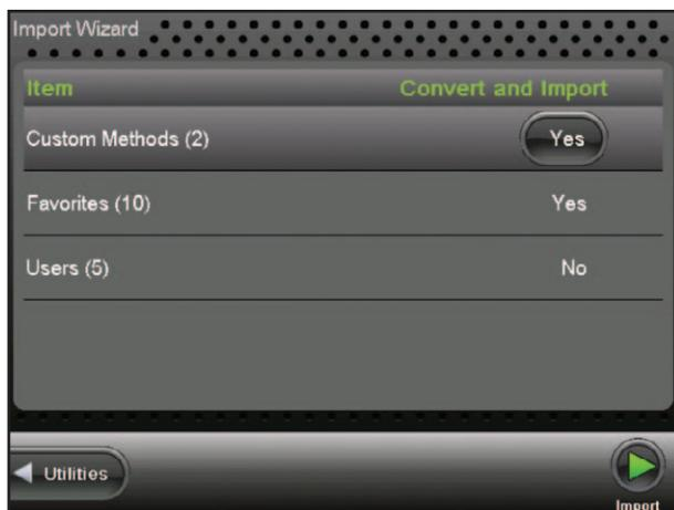
Toggle the Convert and Import buttons to Yes for the files you wish to convert. Then press the Import Run button to convert the selected files. Converting the files allows the user to use the files from controller 61500-01 on 61500-05. The conversion process creates new files and does not delete the originals from the SD card. The methods, Favorites and users are functional on the old and new controller.
