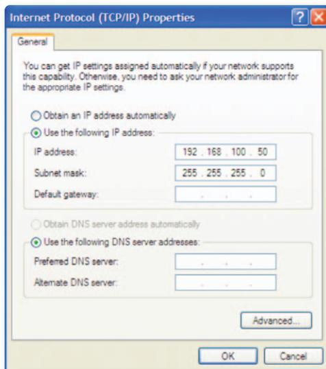
**Step 4.** Select “Use the following IP address” and enter 192.168.100.50 for the IP address and 255.255.255.0 for the Subnet mask. Press the OK button and close all open dialog boxes so the settings take effect.
